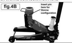
6.1.1. To adjust the trolley jack for each configuration, the head assembly of the lifting arm is moved to the desired position (fig's 4A & 4B) and secured in place with pin. Note pin locations on each configuration.
